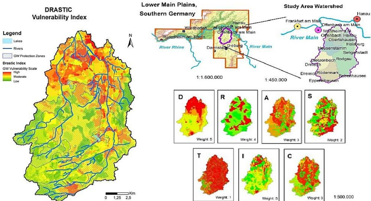
**Figure 1** – The study area location and DRASTIC groundwater intrinsic vulnerability index.
